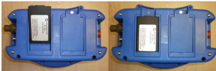
Fig. 5: Installation of Battery Pack into XLTX Transmitter
