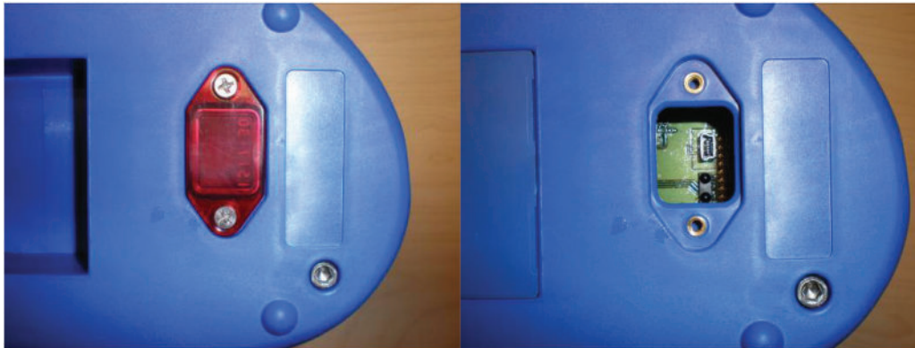
Fig. 12: USB/IR Cover Location and Cover Removal – MLTX2
