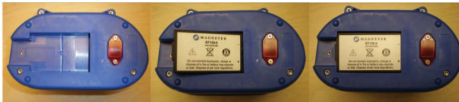
Fig. 6: Installation of Battery Pack into MLTX2 Transmitter
