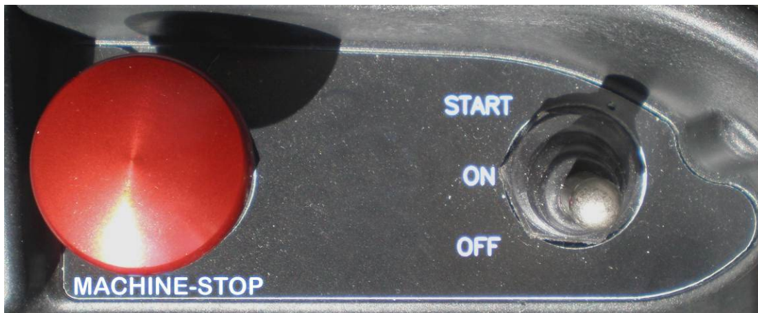
Figure 6: Machine Stop Switch and OFF-ON-START Toggle
