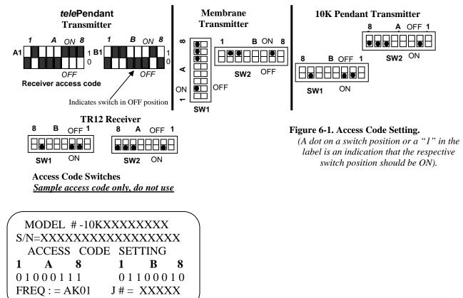
Sample Membrane or Pendant Transmitter Access Code Label Sample access code only do not use
