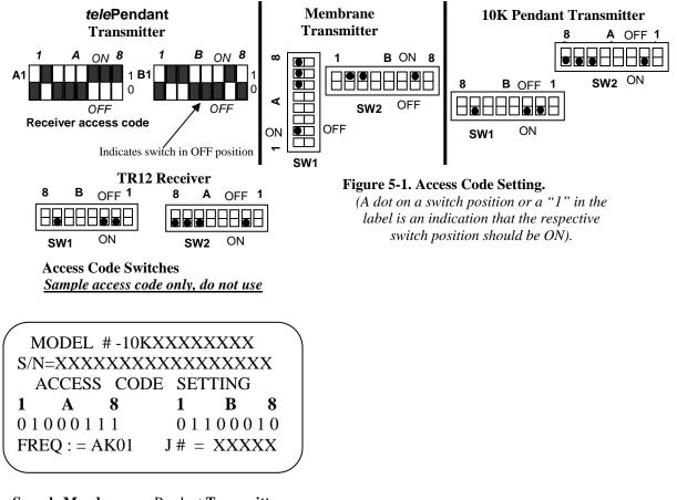
Sample Membrane or Pendant Transmitter Access Code Label Sample access code only do not use
