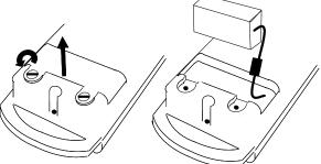
Figure 4-3. telePendant Battery Replacement.
