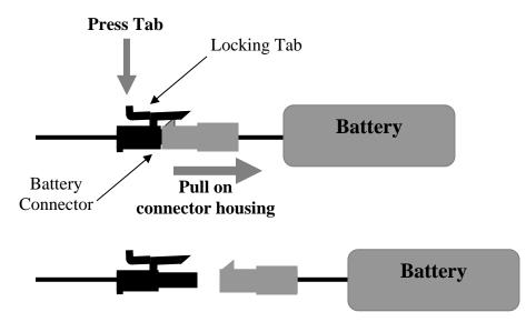
**Figure 4.4 Disconnecting the battery.**
