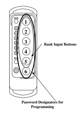
Figure 4-2. Bank and Password Input Buttons.
