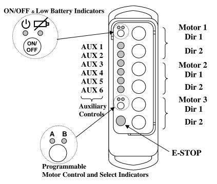
Figure 4-1. 2- and 3-Speed telePendant
