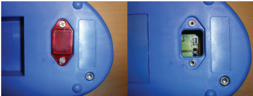
Fig. 12: USB/IR Cover Location and Cover Removal – MLTX2
