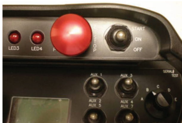
Fig. 14: Machine Stop Switch and OFF-ON-START Toggle Options
