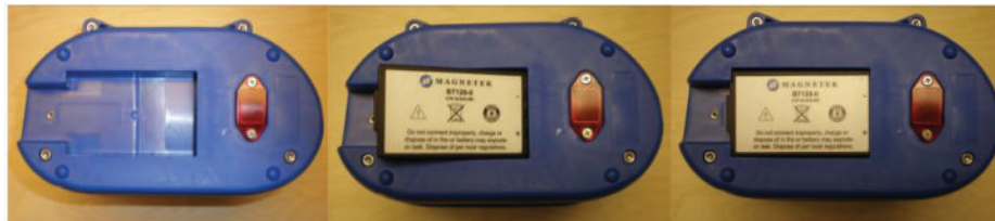
Fig. 6: Installation of Battery Pack into MLTX2 Transmitter
