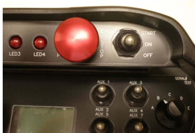
Figure 5: Machine Stop Switch and OFF-ON-START Toggle
