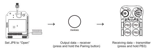
JP8 Short Method (press Pairing button not required): After the transmitter enters the Remote Pairing mode, press and hold PB3 on the transmitter until the Status LED turns to solid green, indicating the pairing is complete. Make sure the transmitter and receiver are within 10 meters from one another and that no other active receivers are nearby during the pairing process. During pairing process, the receiver MAIN relays must be deactivated (relay open).
