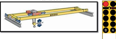
FLEX-EX2-2RS-3M is designed for (1) Bridge and (1) Carrier with independent Controls. This system comes with (1) Bridge receiver and (1) Carrier Receiver. Carriers are controlled by buttons A & B. System uses a Type B transmitter.
