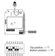
The above dipswitch setting "1 0 0 1 0 0" corresponds to "channel 36" in the system channels table in Section 4.2.10 on page 72.
