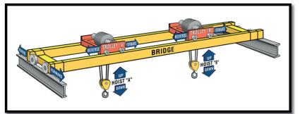
FLEX-EX2-3RS-5M is designed for (1) Bridge and (2) Carriers with independent Controls. This system comes with (1) Bridge receiver and (2) Carrier Receivers. Carriers are controlled by buttons A & B. System uses a Type B transmitter.
