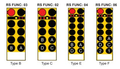
Please note that the Transmitters must be ordered from the Factory with the receiver select Firmware. Standard EX2 transmitters cannot be reprogrammed for RS functionality.
