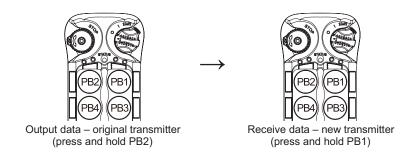
**NOTE:** During remote pairing make sure the distance between the two transmitters is no more than 1 meter.
