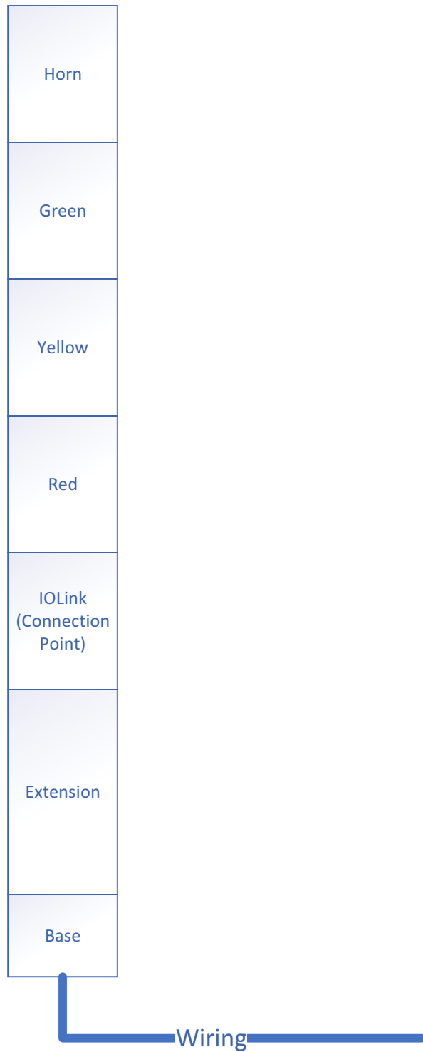
Figure 2-17: Light Stack Install
