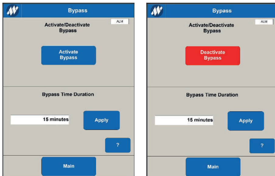
Figure 4-9: Bypass Activated and Deactivated Screens
